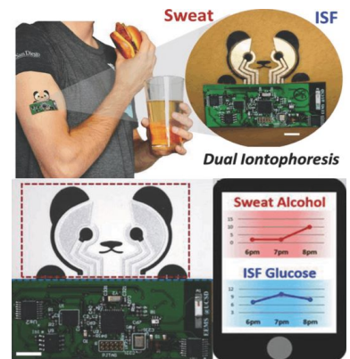
Figure 1.16: Depiction of the wearable iontophoretic biosensor device developed by Kim et al. for glucose and alcohol monitoring on a human subject. A wearable app allows the user to read its glucohol levels. From [65]
