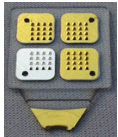
Figure 3.20: Bollella et al.'s Polycarbonate structure of four 4x4 microneedle arrays metalized with gold and silver. From [234]
