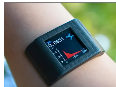
Figure 2.5: The wearable free-standing electrochemical sensing system similar to a smartwatch developed by Zhao et al. [100]. Credit: Yichao Zhao/UCLA [101]
