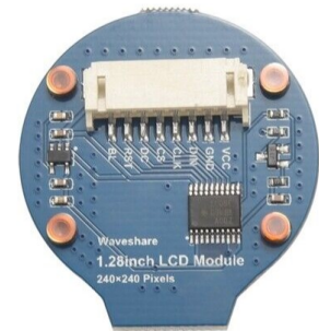
Figure 2.9: Back of module GC9A01, with the four screw slots visible.
