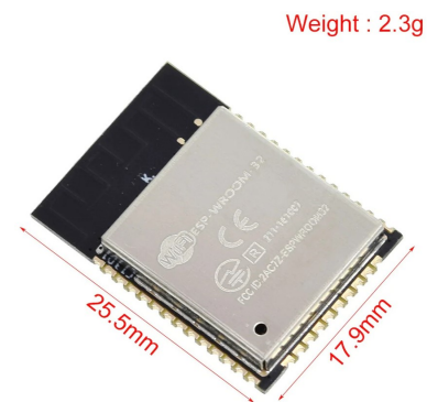
Figure 2.15: ESP32 Wroom dimensions.
