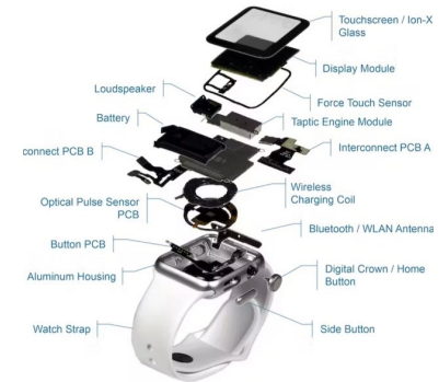
Figure 2.3: Exploded view of the Apple Watch. From [87]
