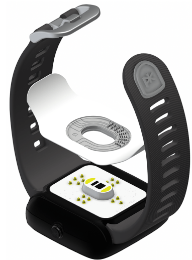
Figure 1.21: Illustration of the Kapsul: the replaceable micro-needles biosensor module for the K'Watch. From [73]
